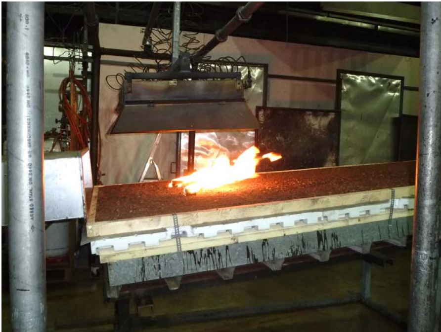
Illustration 3: Approx. one minute after the two incendiary agents were put in place, the flames, fuelled by the airflow from the blower, were up to 50 cm in length (photo shows a build-up with Floraset® FS 50)
