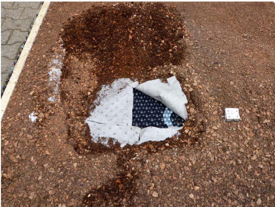
Illustration 4: Despite the fact that shortly after the end of the test the surface temperature of the substrate layer was about 300 °C, no effects of the fire were observed on the filter sheet or the drainage element (photo shows build-up with Floradrain® FD 25).
