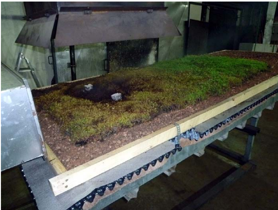
Illustration 6: After the incendiary agents were extinguished, the radiant heat continued to be applied until the end of the 30 minute test. This led to the vegetation drying out across a diameter of about 80 cm.
