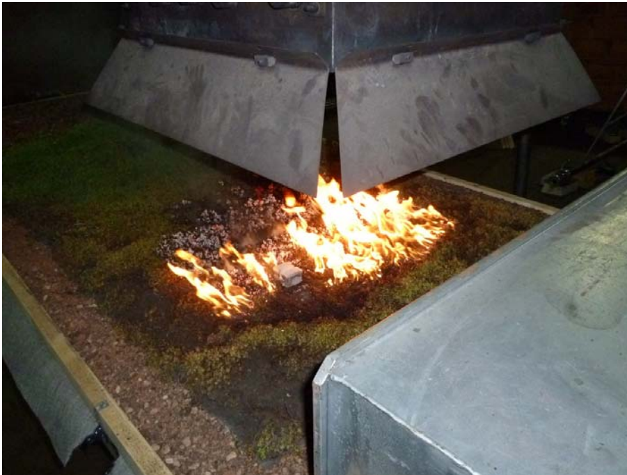
Illustration 7: After the end of the actual test, the dried-out area was set alight using a naked flame applied externally. The fire extinguished of its own accord after 2 minutes. The area of the vegetation mat that was still "damp" was unaffected.
