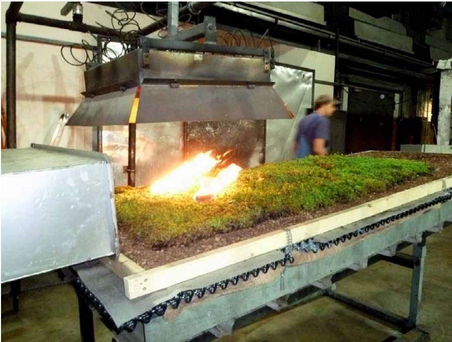
Illustration 5: The test was passed even with a vegetation mat in place; the incendiary agents extinguished after 12 minutes without the vegetation catching fire.
